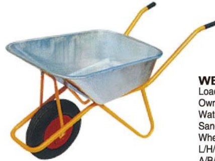
WB6432 Load Capacity(kg):160 Own Weight(kg):15.1 Water capacity(L):72 Sand Capacity(CBF):5 Wheel:3.25-8 L/H/C(mm):1390x530x620 A/B/h(mm):875x595x285
