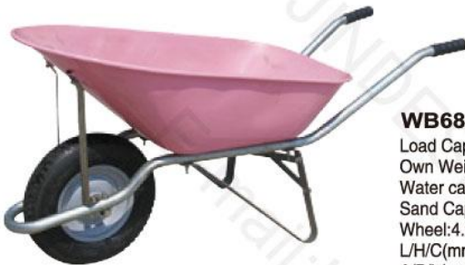
WB6416 Load Capacity(kg):150 Own Weight(kg):14 Water capacity(L):75 Sand Capacity(CBF):5 Wheel:4.00-8 L/H/C(mm):1500x550x600 A/B/h(mm):860x600x285
